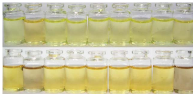
Fig. 3 Color changes of receptors 6 and 7 upon addition of anions. [ 6 ] = [ 7 ] = 3 \times 10^{-5} M in DMSO; 6 + 10 equiv. anion (top), 7 + 5 equiv. anion (bottom). From left to right: none, \text{F}^- , \text{Cl}^- , \text{Br}^- , \text{I}^- , \text{HSO}_4^- , \text{H}_2\text{PO}_4^- , \text{NO}_3^- , \text{CH}_3\text{COO}^- .
